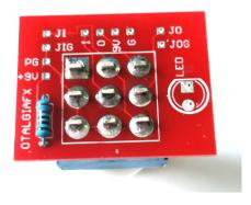
**STEP 3**— Solder the Power supply and Jack Input and Output wires
