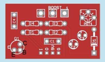
The transistor will need to be orientated correct and match the placement image marked on the PCB. If you intend to use a transistor that differ from the build list then please be aware than the Collector, Base and Emitter legs may be in a different order. The pinout legs of different transistors can be found by referring to their technical data sheets on the Web.
