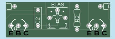
The transistors will need to be orientated correct and match the placement image marked on the PCB. If you intend to use transistors that differ from the build list then please be aware than the Collector, Base and Emitter legs may be in a different order. The pinout legs of different transistors can be found by referring to their technical data sheets on the Web.
