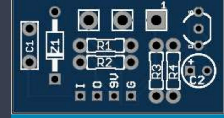
"A nice clean Mosfet booster based on a popular crackling boutique pedal"
